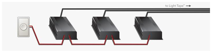
Adjust various power supplies with different Light Tape® lamp loads using the same dimming controller.
