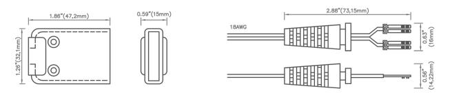
Small Connector Cap, with 3M™ rubber mastic lining. Suitable for 0.25" (6.35mm) Light Tape®. Supplied with standard connector, integrated strain relief, Nicomatic Crimpflex™ 11612-12 soldered contact pins, with 6ft (1.8m) black lead.
