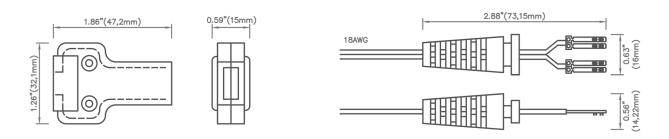
Crimpflex™ DFM locked/semi-locked housing. Suitable for 0.25" (6.35mm) - 0.5" (12.7mm) Light Tape®. With Nicomatic Crimpflex™ 10025-1X soldered contact pins. Please note, micro connections are made to order, please contact us to determine application suitability. 0.25" (6.35mm) model specifications shown.
