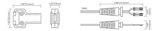
Crimpflex<sup>™</sup> DFM locked/semi-locked housing. Suitable for 0.25" (6.35mm) - 0.5" (12.7mm) Light Tape<sup>®</sup>. With Nicomatic Crimpflex<sup>™</sup> 10025-1X soldered contact pins. Please note, micro connections are made to order, please contact us to determine application suitability. 0.25" (6.35mm) model specifications shown.
