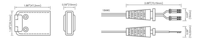
Small Connector Cap, with 3M<sup>™</sup> rubber mastic lining. Suitable for 0.25" (6.35mm) Light Tape<sup>®</sup>. Supplied with standard connector, integrated strain relief, Nicomatic Crimpflex<sup>™</sup> 11612-12 soldered contact pins, with 6ft (1.8m) black lead.
