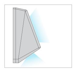
Black PVC unit for aisle chair numbering or signage system. For use with 1" Light Tape® on sign combined with OSRAM LED module on bottom for aisle and tread illumination. Customized with any sign or number in black adhesive vinyl.
