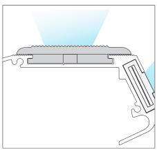
ABS cover / Polycarbonate enclosure unit for row step numbering or signage system. For use with 3/4" Light Tape®.
