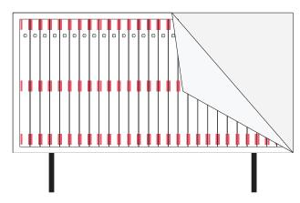
The 'base' vinyl layer that will support the Light Tape® OOH Panel System. This layer is printed with a layout template that guides the installation of Light Tape® panels using industrial Velcro denoted in red.
